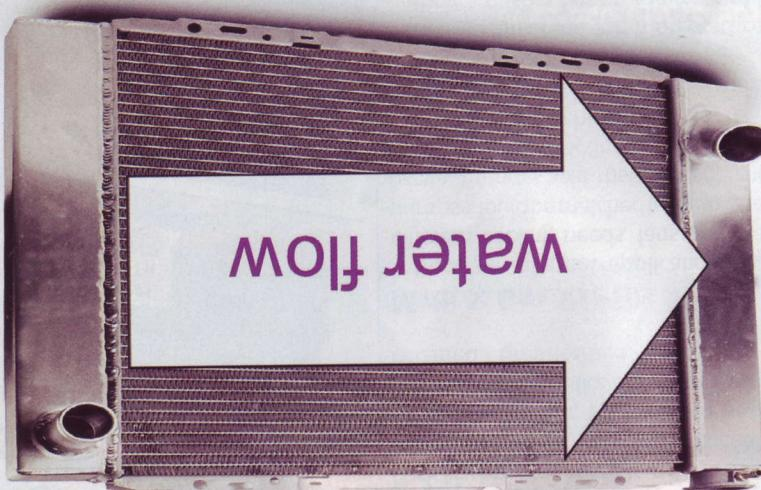
"By running a higher pressure system, we are effectively squeezing the suspended air molecules within the water itself and if we can do that, we can have a better contact area and a better heat exchange," Brenner explained.
